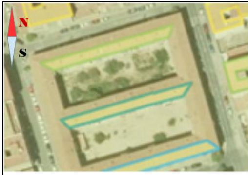
Fig.3 Example of pitched rooftops oriented north-south. Only the highlighted area has been considered for the rooftop surface estimation.
