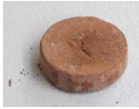
Figure 41: Second LMS sample obtained with microwave sintering.
