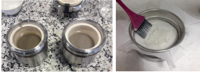
Figure 15: Image of the grinding bowls after milling on the left and sieving of the powder on the right.
