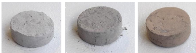
Figure 35: LHS (left), LMS (center), MGS (right) green body made with milled simulants.
