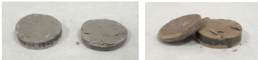
Figure 34: Broken LMS (left) and MGS (right) green body made with milled simulants.
