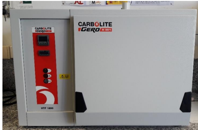
Figure 17: Carbolite Gero high temperature furnace used for conventional sintering.
