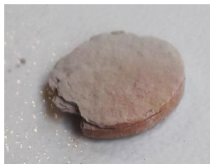
Figure 42: LHS sample obtained with microwave sintering.
