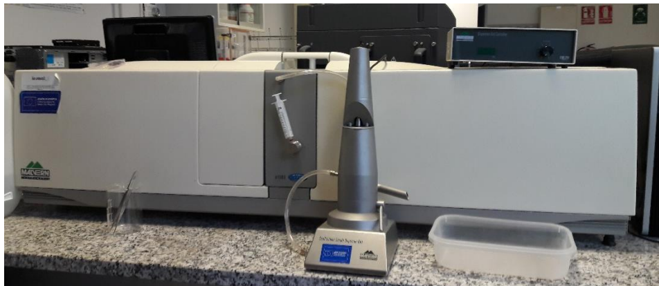
Figure 23 : Malvern Panalytical Mastersizer 2000, with the dispersal unit in the centre.
