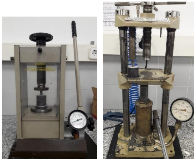
Figure 16: Image of the uniaxial press on the left, and of the demoulding press on the right.
