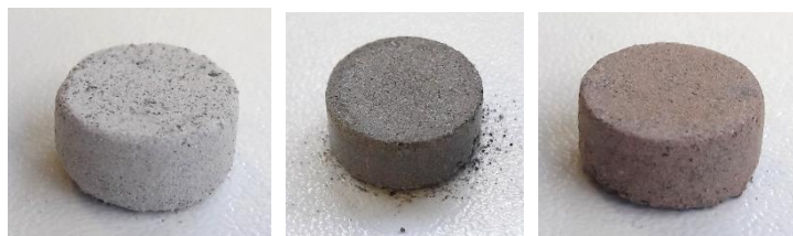
Figure 36: LHS (left), LMS (center), and MGS (right) green body made with unmilled simulants.
