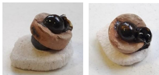
Figure 40: First LMS sample obtained with microwave sintering.
