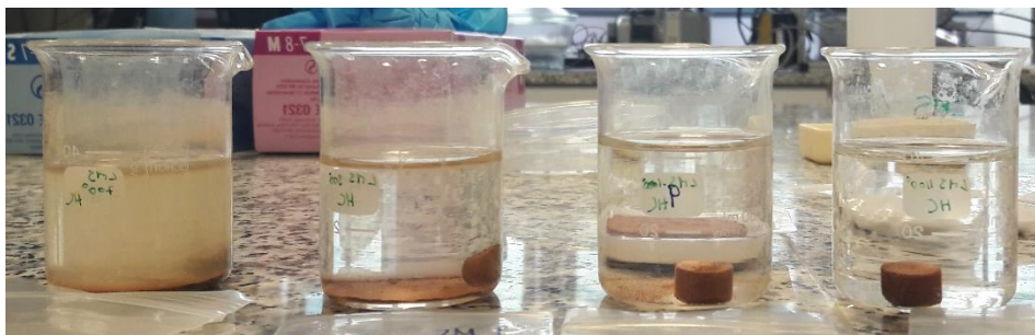
Figure 37: Samples made of raw LMS and heated 3 hours in distilled water. They were sintered in conventional oven at (from left to right) 700, 900, 1000 and 1100 °C.
