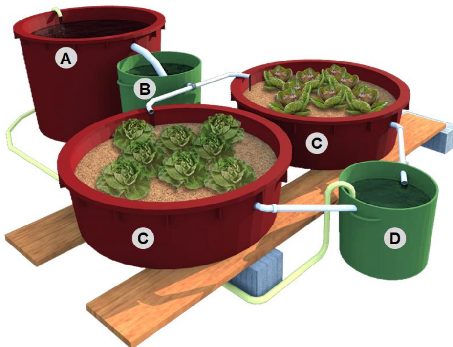
Figure 4.1. Rendering of the aquaponic unit. A, main tank for fish (500 L); B, sedimenter; C, tanks for vegetables/biofilters (275 L); D, storage tank for water collection (50 L) and pumping to A tank.
