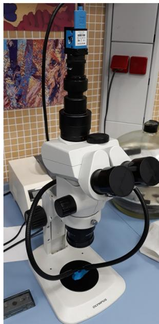
Figura IV- 23. Estereomicroscopio Olympus SZX7.
