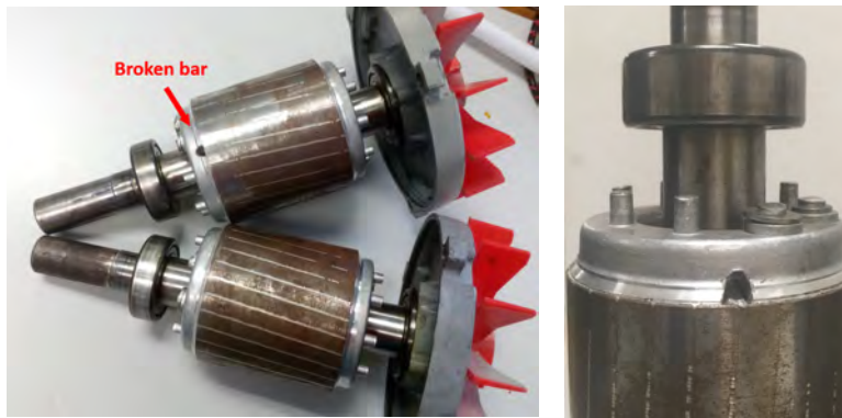
Figure 7: Experimental motor of Appendix A with a provoked broken bar. Comparison with a healthy rotor (right) and close view of the bar breakage, at the junction with the end ring (right).
