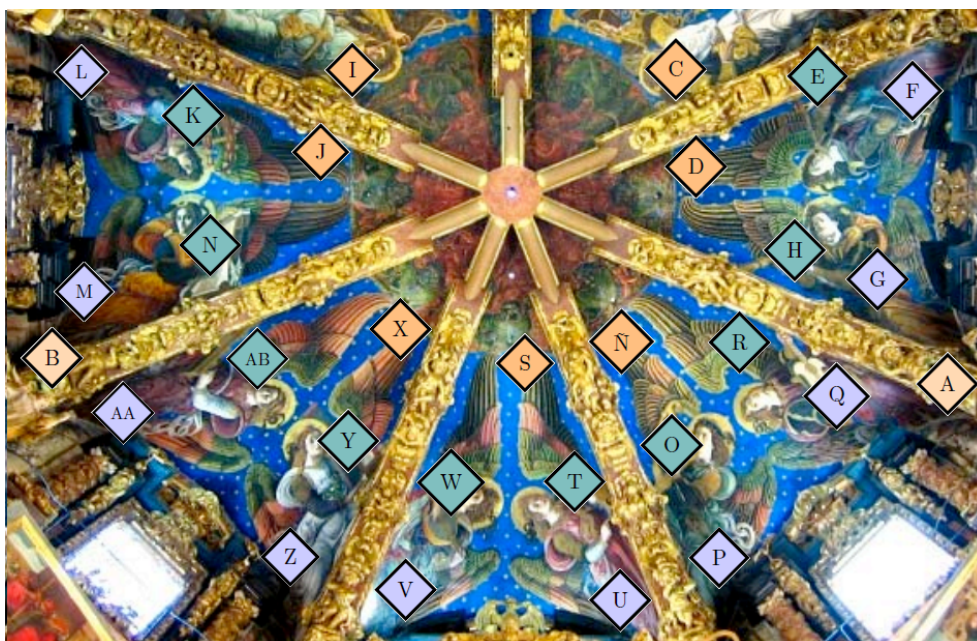
Figure 2.1: Approximate location of the probes and sensors at the apse vault of the cathedral of Valencia. Details of the installation of the probes and a scheme depicting the installation of probes in the frescoes can be seen in [7] and [6]. The image shows the position of the 29 probes for monitoring the relative humidity (RH) of the indoor atmosphere, displayed in different colors according to their position. Seven probes were located on the ribs (orange), two at the cornice (light orange), ten on the walls below the severies (purple), and ten probes on the frescoes (green).
