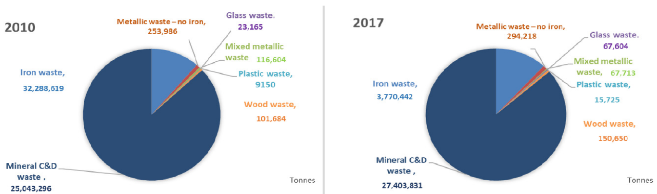
Figure 10. C&D waste material prepared to be recycled (tonnes). Source: Own elaboration from ISPRA data.
