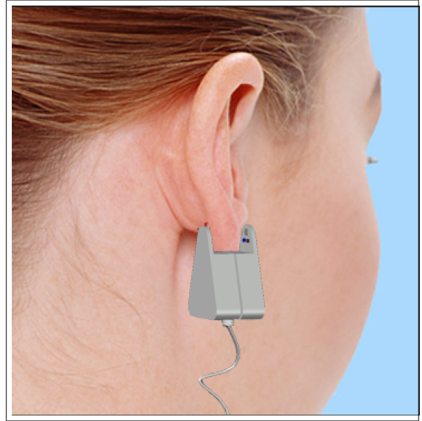
Fig. 3. Example of the wired prototype of the sensor, placed in the ear lobe
