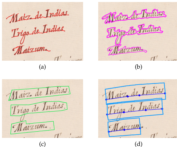
Figure 4.1: Example of different ways to define the polygon that best surrounds the text line. a) a cumbersome detailed polygon, b) a detailed polygon, that is still cumbersome, c) an easy to define sketchy polygon, d) a simple polygon defined from the baselines.
