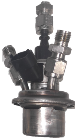
Figure 2.13: Liquid-cooled UWS injector.
