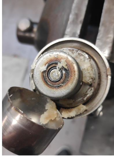
Figure 2.14: Example of deposit formation in a commercial nozzle.
