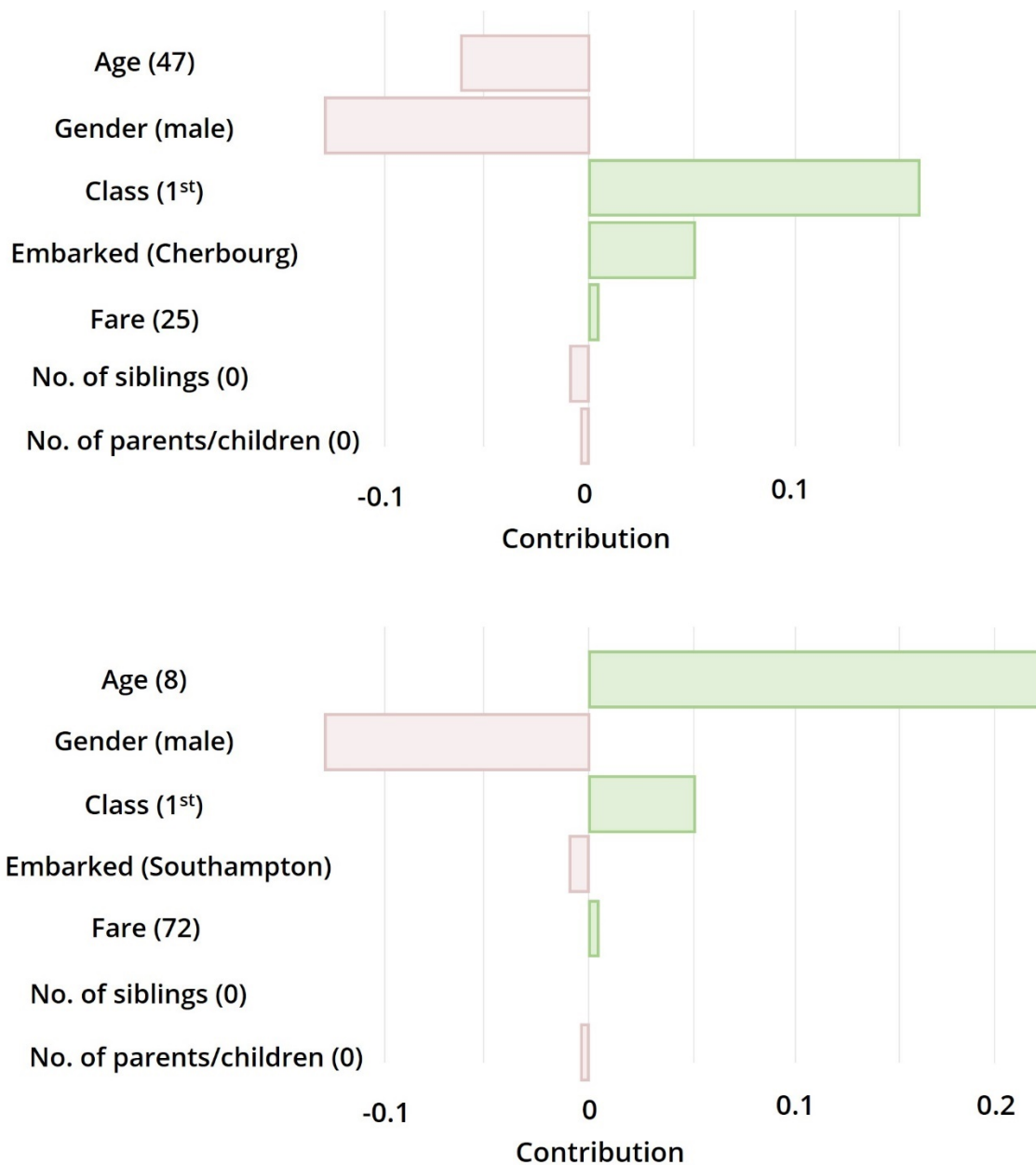
Figure 70. Example of the predictors' contribution of two Titanic passengers. Green and purple bars represent SHAP values. In this example, the young age of 8 increases the chances of survival, contrary to the negative contribution of the age of 47.
