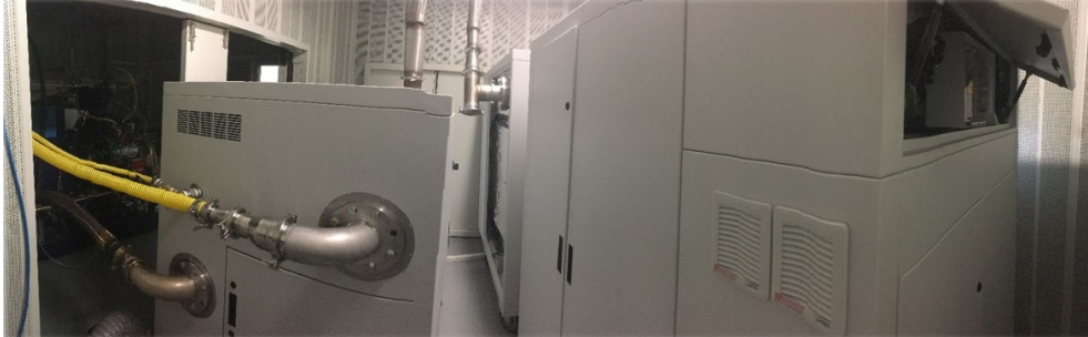
Figure 3.3: MEDAS connected to the temperature module and to the engine.
