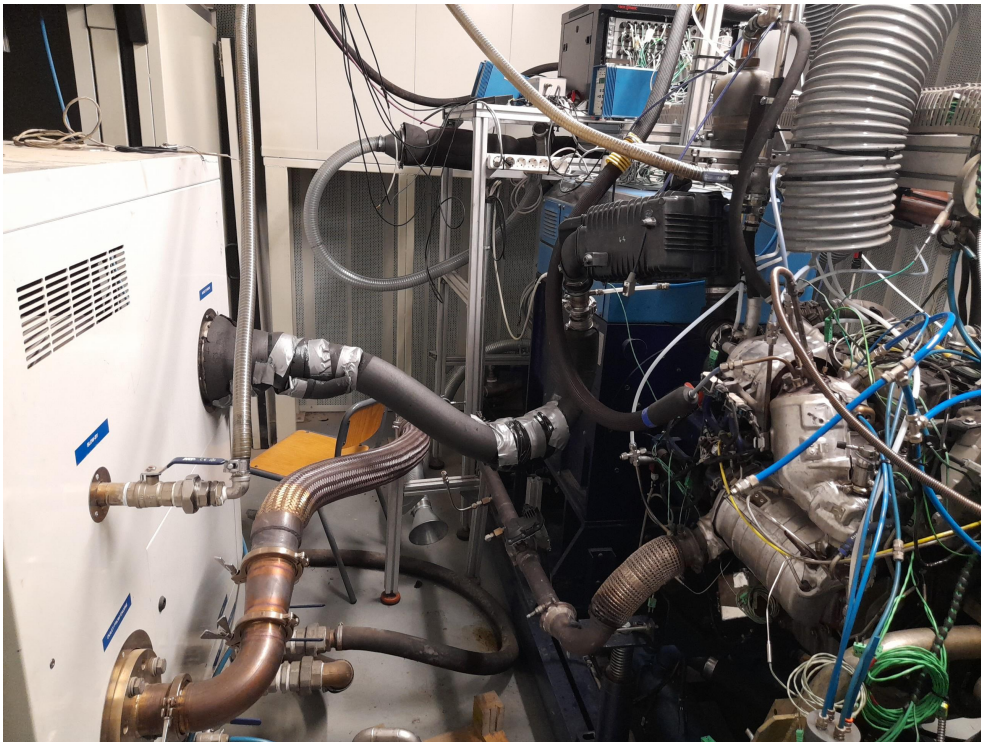
Figure 3.4: MEDAS connection with the engine.
