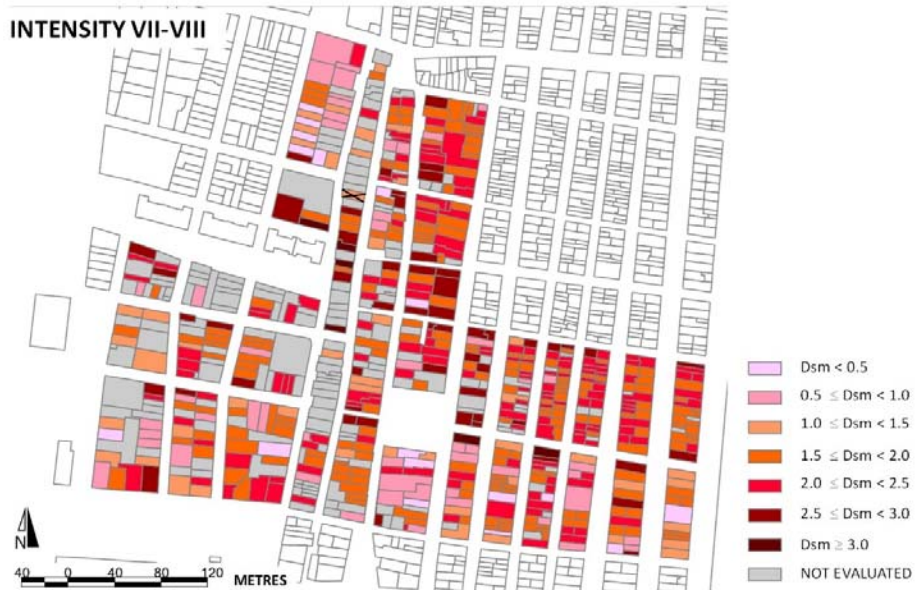
Figure 14 Mean damage index distribution (Dsm) for intensity VI, VII and VII-VIII
