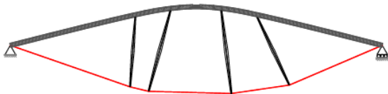
Figure 8: Example of a generic structure with n = 5 elastica sections shaped with the sequential method
