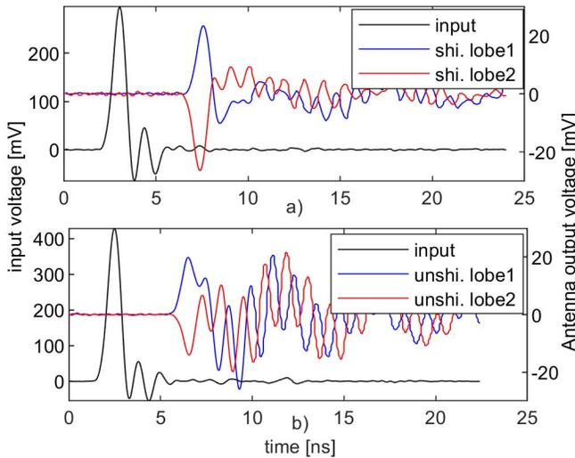
Fig. 8. UHF pulse measured with symmetric lobes in a) shielded and b) unshielded, magnetic antenna.
