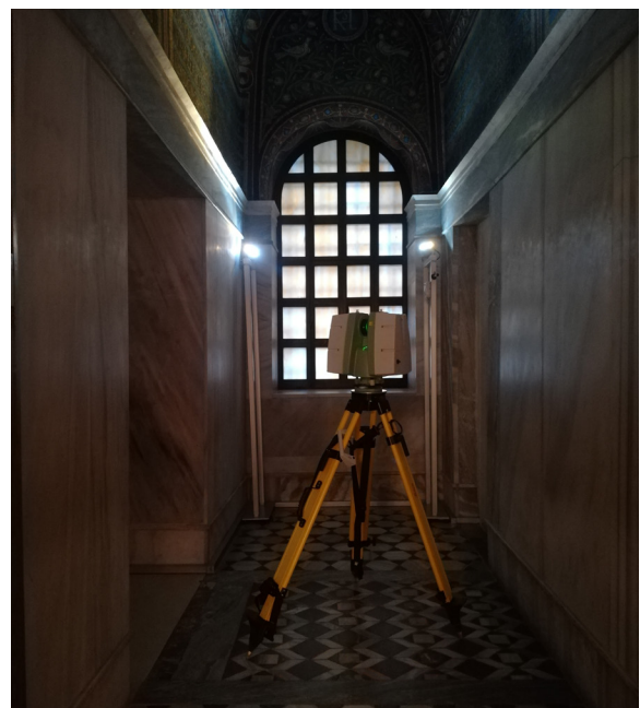
Fig. 27_ Leica ScanStation C5 in the vestibule of the chapel
