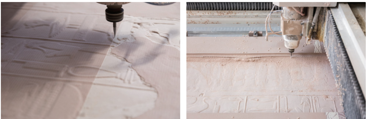
Fig. 10_ Carving of the Seti I's tomb to create a physical replica. Lowe, 2017
