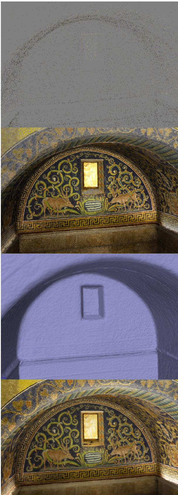
Fig. 22_ Mausoleum of Galla Placidia. Digital photogrammetry workflow from point cloud to textured mesh
