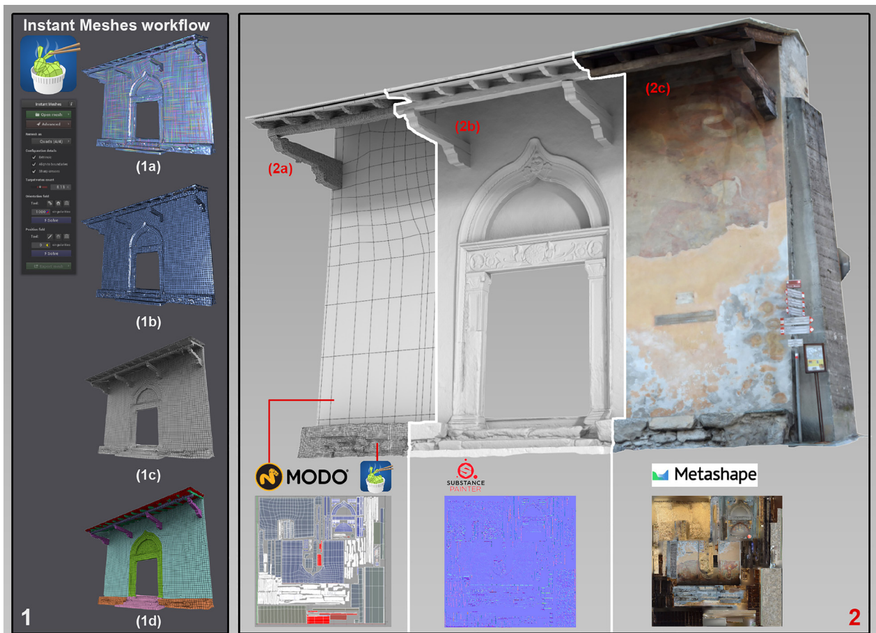
Fig. 59. Optimising workflow for a 3D reality-based model. From Bertacchi S. et al. (2021)
