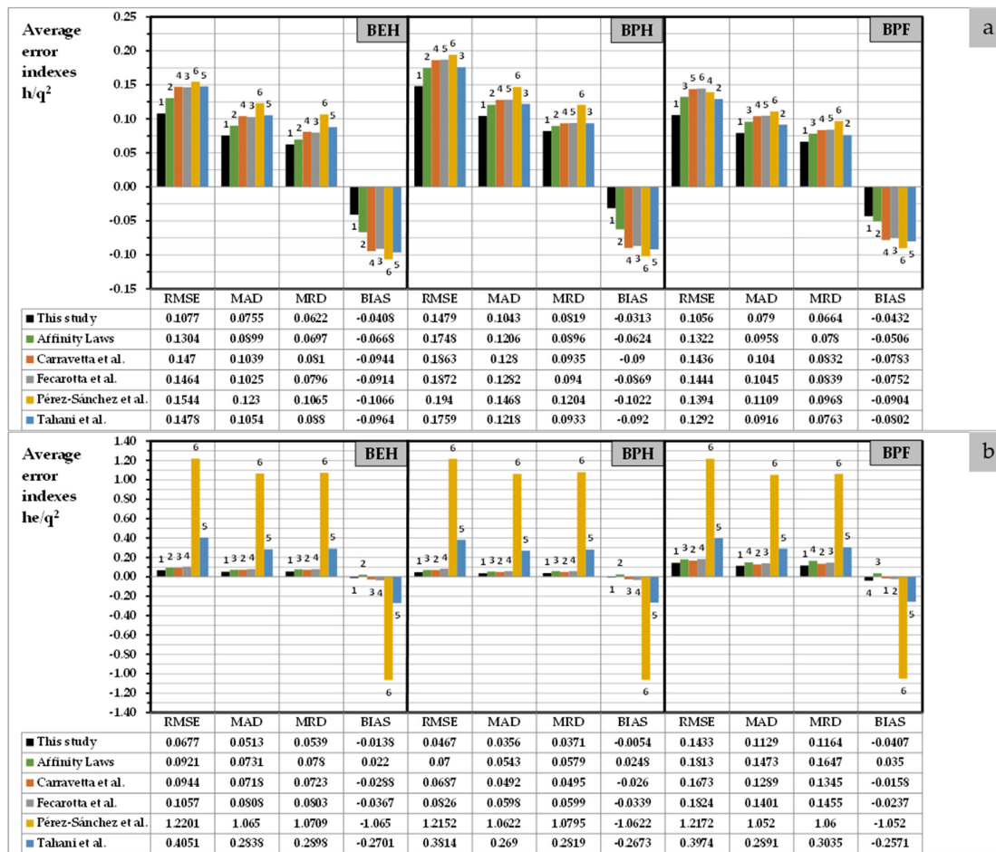
Figure 4. (a) Error indexes for the different methods applied to h/q^2 ; (b) error indexes for the different methods applied to he/q^2 .
