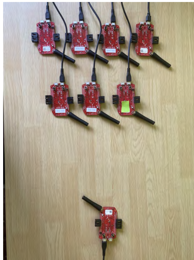
Figure 6. Testbed deployment using Zolertia RE-Mote platform.
