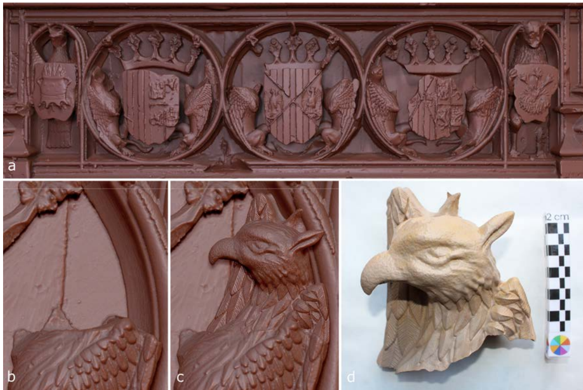
Fig. 5 (a-d). 3D reconstruction of the Griffins. a) Digital model of the missing areas of the tondos. b) Detail of the area of a tondo without volume. c) Detail of the digitally modelled area. d) Prosthesis printed with SLA and treated chromatically.
