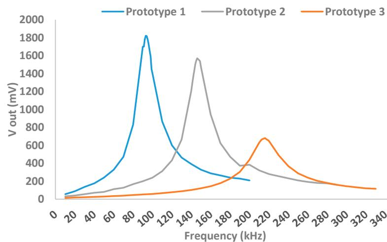
Figure 6. Resonance frequency obtained for each prototype.
