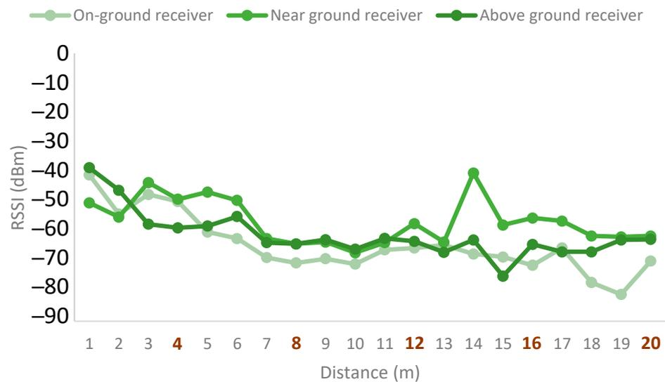
Figure 15. Emitter at height of 1 m.
