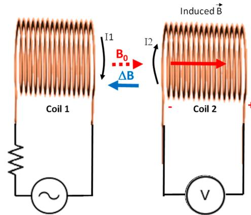
Figure 3. Principle of operation for our developed sensor.
