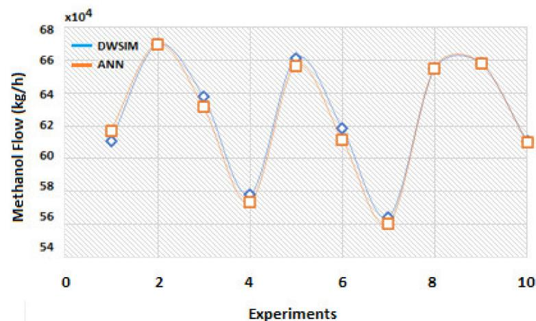
**Figure 10.** Comparison between observations (DWSIM-blue) and predictions of ANN (orange) methanol flow.
