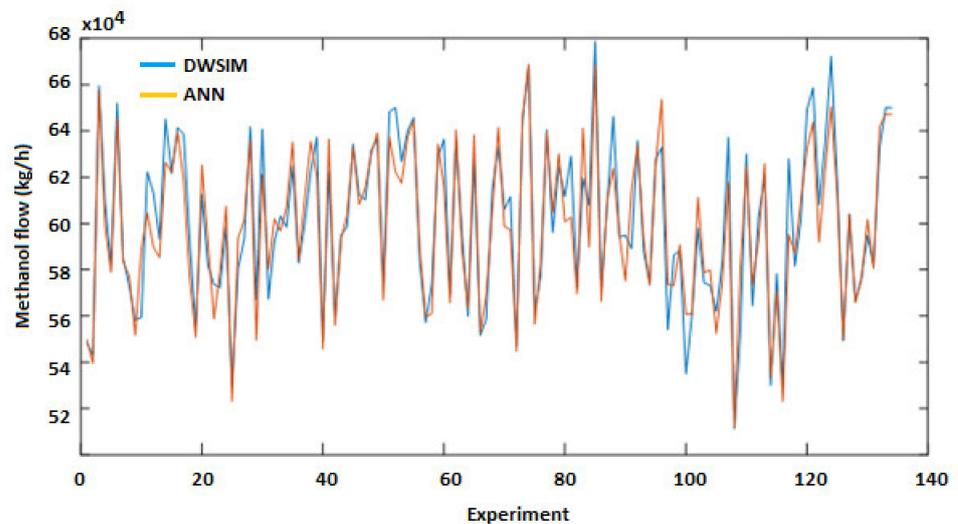
Figure 9. Comparative graph of the experimental data (DWSIM) and ANN predictions regarding methanol flux (kg/h).
