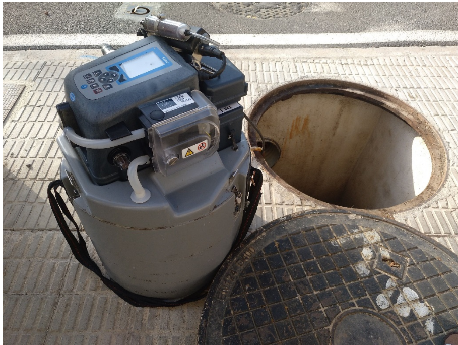
Figure 6. Example of automatic sampler used for monitoring.
