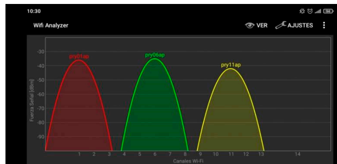
Figure 11. WiFi interference generators. Each colour shows an individual WiFi Network and its relation to signal strength and WiFi channel occupation.
