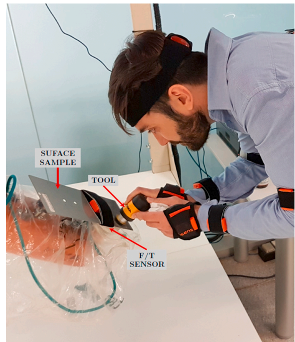
Fig. 18. Setup used for measuring the forces exerted by the expert on the workpiece surface while performing the surface treatment task: an F/T sensor, a polishing tool and a sample surface with defects.
