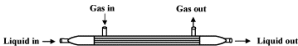
Figure 5: Schematic of Longitudinal Flow Module.
