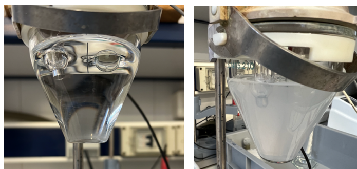
Figure 5. 8 – Aqueous electrolytes containing (a) 1 M ZnCl 2 (transparent) (b) 0.25 M ZnCl 2 (cloudy).
