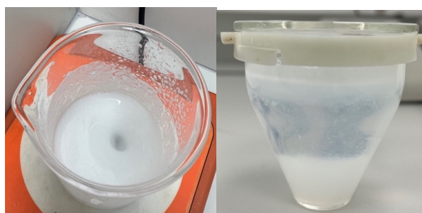
Figure 5.20 – Experimental pictures of \text{Zn}(\text{OH})_2 precipitation in a 100 ml 1 M NaOH – 1M \text{ZnCl}_2 solution
