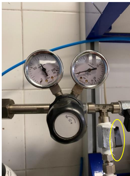
Figure 9.20: Pressuring the System
