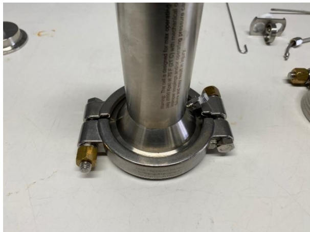
Figure 9.7: Tightening of Bottom of Cell Body
