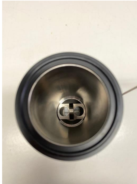
Figure 9.10: Magnetic Stirrer in Place
