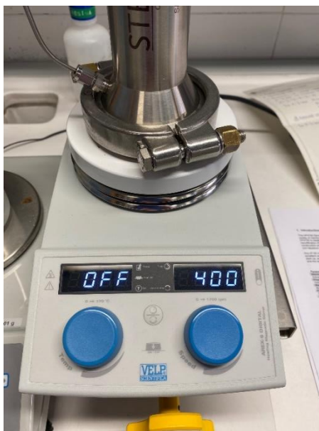
Figure 9.17: Magnetic Stirring Initiated
