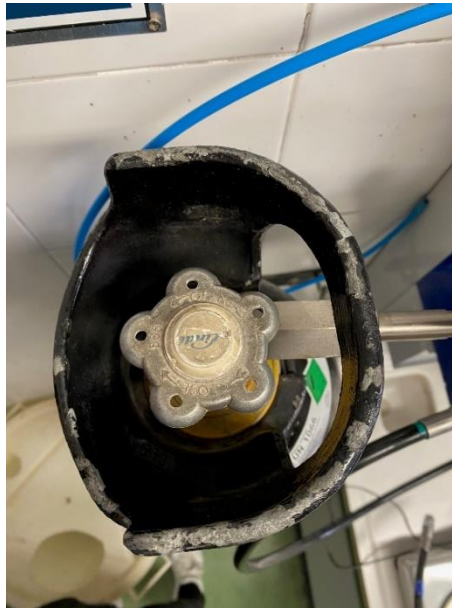
Figure 9.19: Opening of Nitrogen Tank
