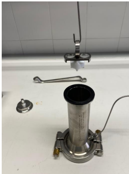
Figure 9.9: Lowering of Magnetic Stirrer
