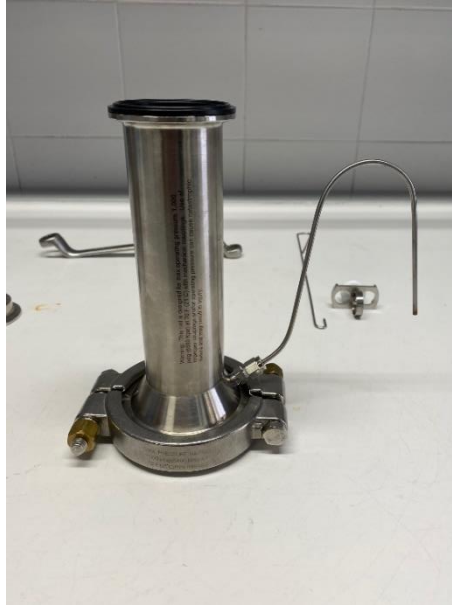
Figure 9.8: Attachment of Permeate Tube
