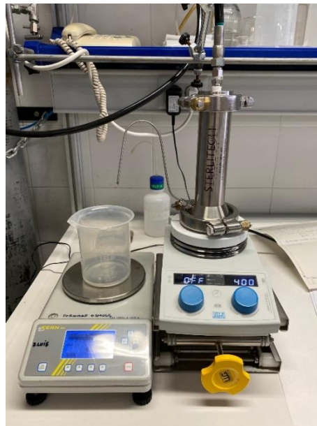
Figure 9.15: Cell and Magnetic Stirrer Placement
