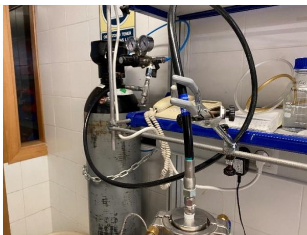
Figure 9.13: Connecting Cell to Pressurised Nitrogen
