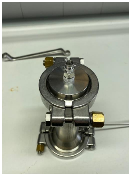
Figure 9.12: Tightening of Top Cell Section
