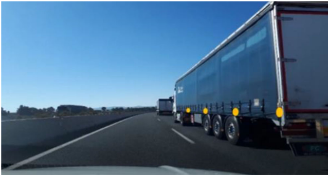
FIGURE 13 Dynamic lighting warning system
