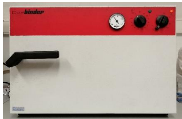
Figure 14. Drying Oven used for moisture content determination [18].
