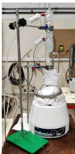
Figure 18. Setup for extractive determination [18].
