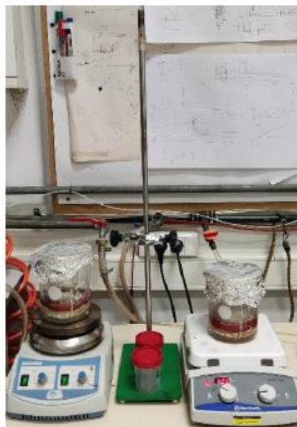
Figure 17. Setup for lignin and hemicellulose determination [18].
