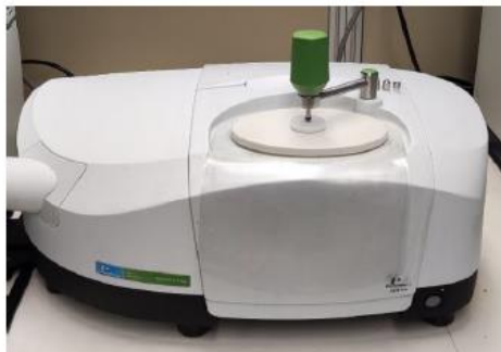
Figure 16. Perkin Elmer Spectrum Spectrometer [18].
