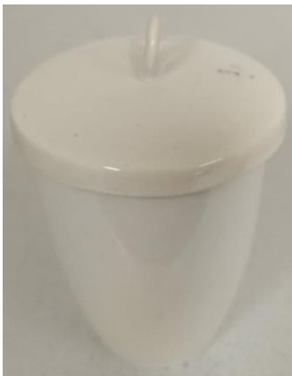
Figure 15. Crucible and lid used for proximate analysis [18].
