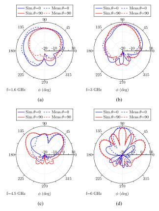
**FIGURE 10.** Simulated (solid) and Measured (dashed) radiation pattern when Port P3 is excited. Plane  $\theta = 0^{\circ}$  (blue) and  $\theta = 90^{\circ}$  (red) at: a) f = 1.6 GHz, b) 3 GHz, c) 4.5 GHz and d) 6 GHz.
