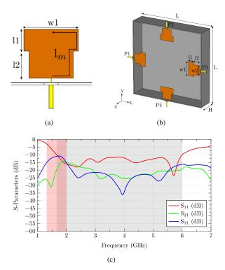
FIGURE 1. a) T-shaped monopole; b) Initial design with the squared cavity; c) S-Parameters of the initial design, where  $S_{21} = S_{41}$  and  $S_{31} = S_{42}$ . Note that red area highlights the band with high coupling levels (from 1.35 to 2 GHz), whereas grey area shows the operating bandwidth (from 1.55 to 6 GHz). Dimensions are detailed in Table 1.
