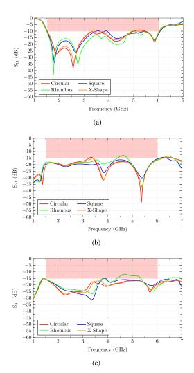
**FIGURE 7.** a)  $S_{11}$  of the four analyzed designs, b)  $S_{21}$  of the four analyzed designs and c)  $S_{31}$  of the four analyzed designs. Red area (values in the impedance bandwidth from 1.55 to 6 GHz in which minimum matching( $S_{11}$ ) or coupling ( $S_{21}$ ,  $S_{31}$ ) is not satisfied).
