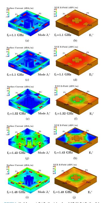
**FIGURE 5.** Modal current distribution  $J_n'$  and modal field distribution  $E_n'$  of the initial design at modal resonance  $f_0$ . Instantaneous magnitude: a)  $J_1'$ , b)  $E_1'$ , c)  $J_2'$ , d)  $E_2'$ , e)  $J_3'$ , f)  $E_3'$ , g)  $J_4'$ , h)  $E_4'$ , i)  $J_5'$  and j)  $E_5'$ .
