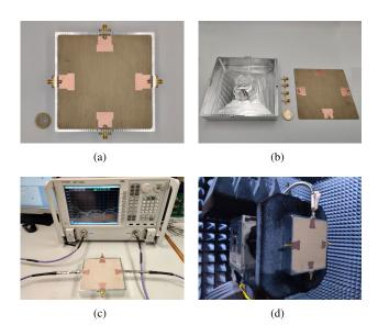
FIGURE 8. a) Fabricated Antenna b) Dissembled antenna c) Antenna set-up for the measurement with the network analyzer and, d) Antenna set-up for the measurement in the anechoic chamber.
