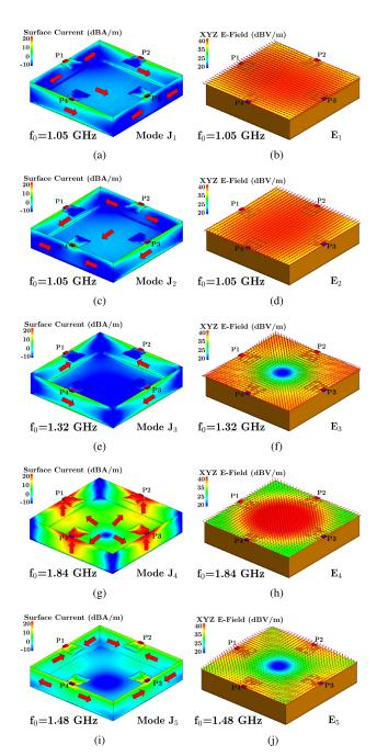
**FIGURE 3.** Instantaneous magnitude of the modal current distribution  $J_n$  and modal field distribution  $E_n$  at modal resonance  $f_0$  of the initial design: a)  $J_1$ ; b)  $E_1$ ; c)  $J_2$ ; d)  $E_2$ ; e)  $E_3$ ; g)  $E_3$ ; g)  $E_4$ ; h)  $E_4$ ; i)  $E_5$  and j)  $E_5$ .
