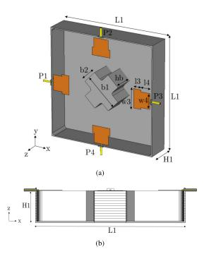
FIGURE 4. a) Overall view of the antenna including the four monopoles coloured in orange and the square open cavity with the X-shaped block coloured in grey. b) Side view of the design (XZ-plane). Dimensions are detailed in Table 2.
