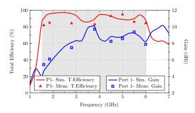
FIGURE 11. a) Total Efficiency (red-left axis) and Gain (blue-right axis) of port P1. Grey area (operating band 1.55-6 GHz).
