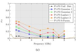
FIGURE 13. a) Analyzed angular distributions: Gaussian 1 (6), Gaussian 2 (7), Laplace 1 (8) and Laplace 2 (9). b) ECC between P1 and P2 and c) ECC between P1 and P3.
