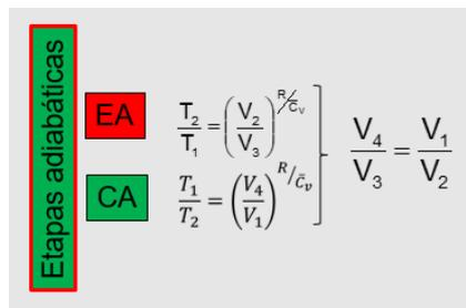
**EA**  $\frac{T_2}{T_1} = \left( \frac{V_2}{V_3} \right)^{R/C_v}$
