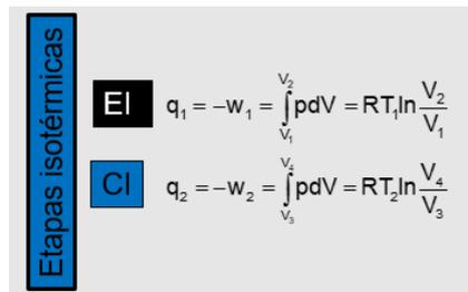
**EI**  $q_1 = -w_1 = \int_{V_1}^{V_2} p dV = RT_1 \ln \frac{V_2}{V_1}$
