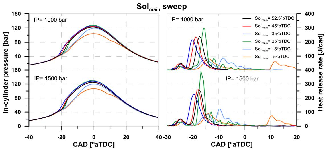
Figure 3. Temporal evolution of the in-cylinder pressure and the HRR for the different  $SoI_{main}$  timings and injection pressures.
