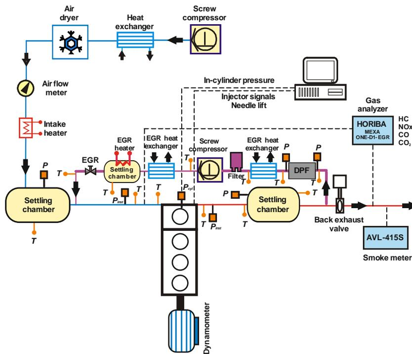
Figure 1. Scheme of the test bench.
