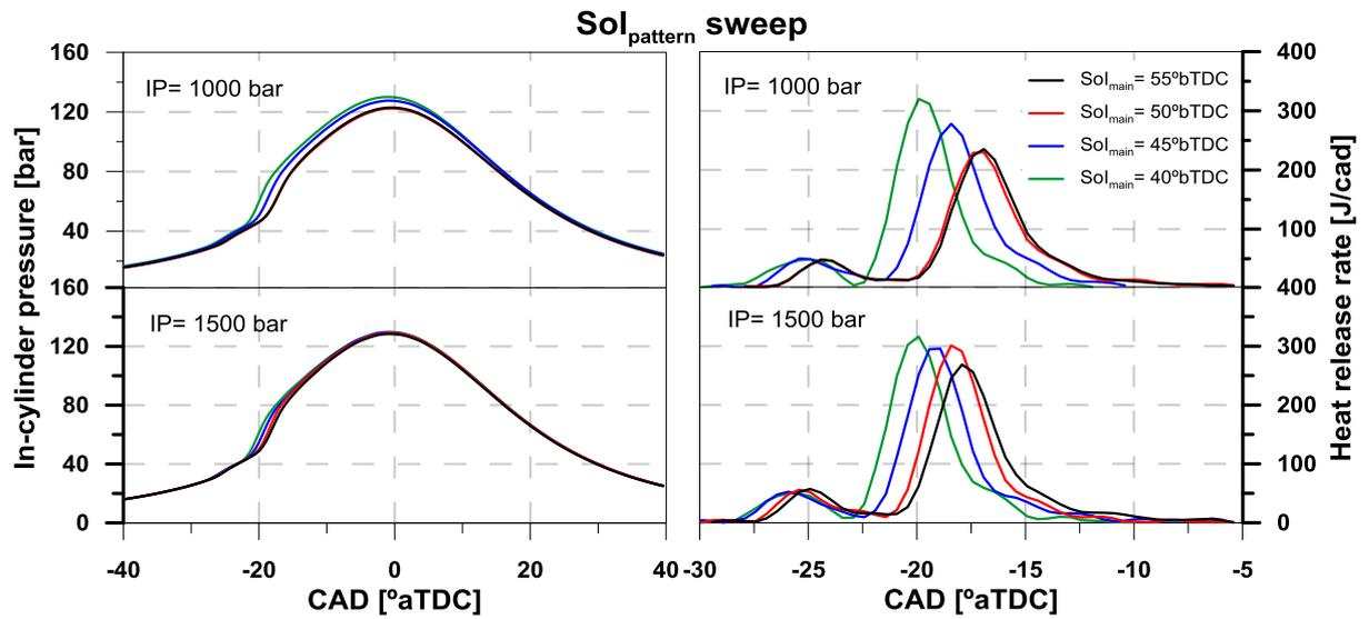
Figure 2. Temporal evolution of the in-cylinder pressure and the HRR for the different injection pattern timings and injection pressures.
