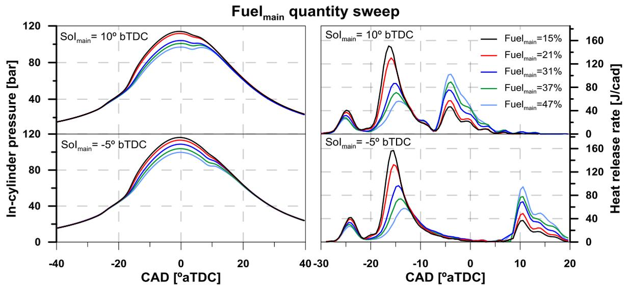
Figure 4. Temporal evolution of the in-cylinder pressure and the HRR (bottom) for the different fuel injection main quantity at two  $Sol_{main}$  timings tested.
