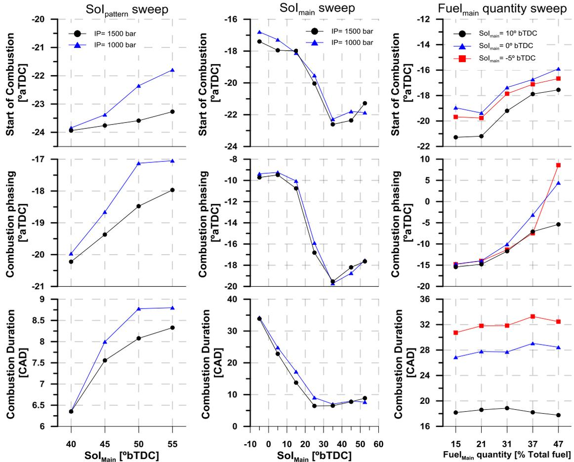
Figure 5. Start of Combustion, combustion phasing and combustion duration for the three studies.
