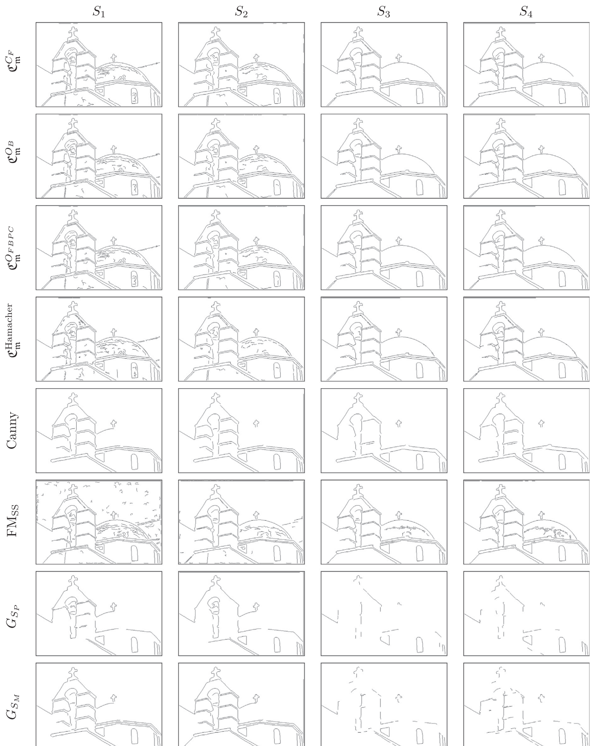
Fig. 7. Visual comparison of the different edge images obtained when applying the proposed functions in Table 1 along with methods from the literature as Canny, FM_{SS} , G_{SP} , G_{SM} .
