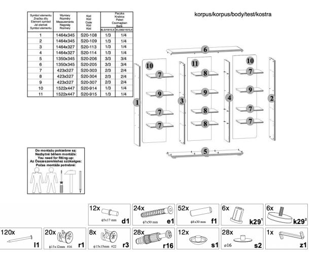
Figure 29.Assembly instructions for ELO/15/13,5 (Source: BRW Sp. z o. o)
