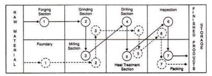
Figure 3. Process or Functional Layout (Source: https://www.yourarticlelibrary.com)
