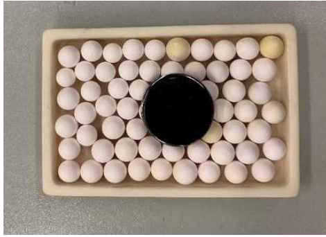
Figure 14: Support plate for the samples filled with Al_2O_3 particles
