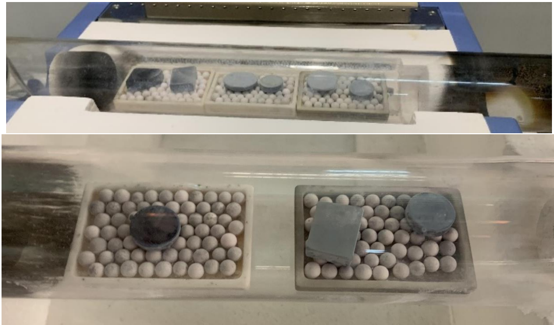
Figure 55: Results of Ti-6Al-4V alloys after heat treatment
