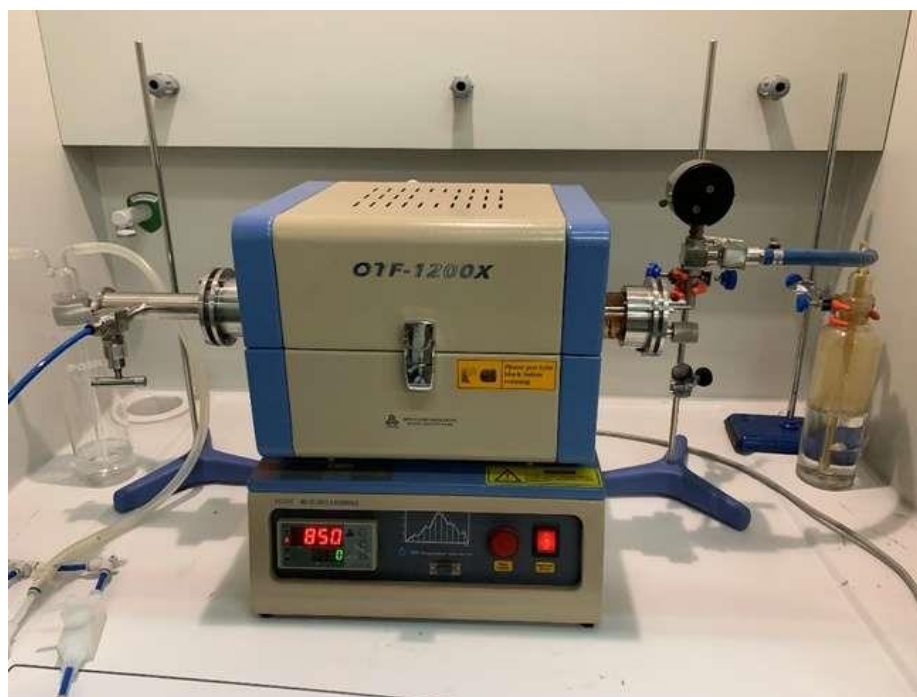
Figure 11: The furnace with the reactor and the 2 bottles (left acetone and right water)
