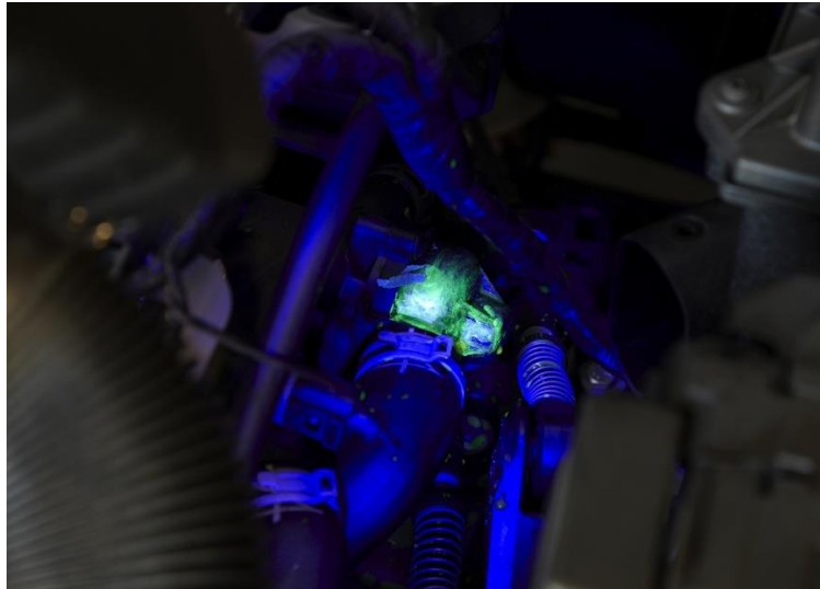
Figure 10: Example of the use of UV dye in a car engine (Coolant System Leak Detection Dye, 2022)
