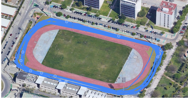
Fig. 2: All these laps were run over the same line. The deviations in the measure are noticeable
