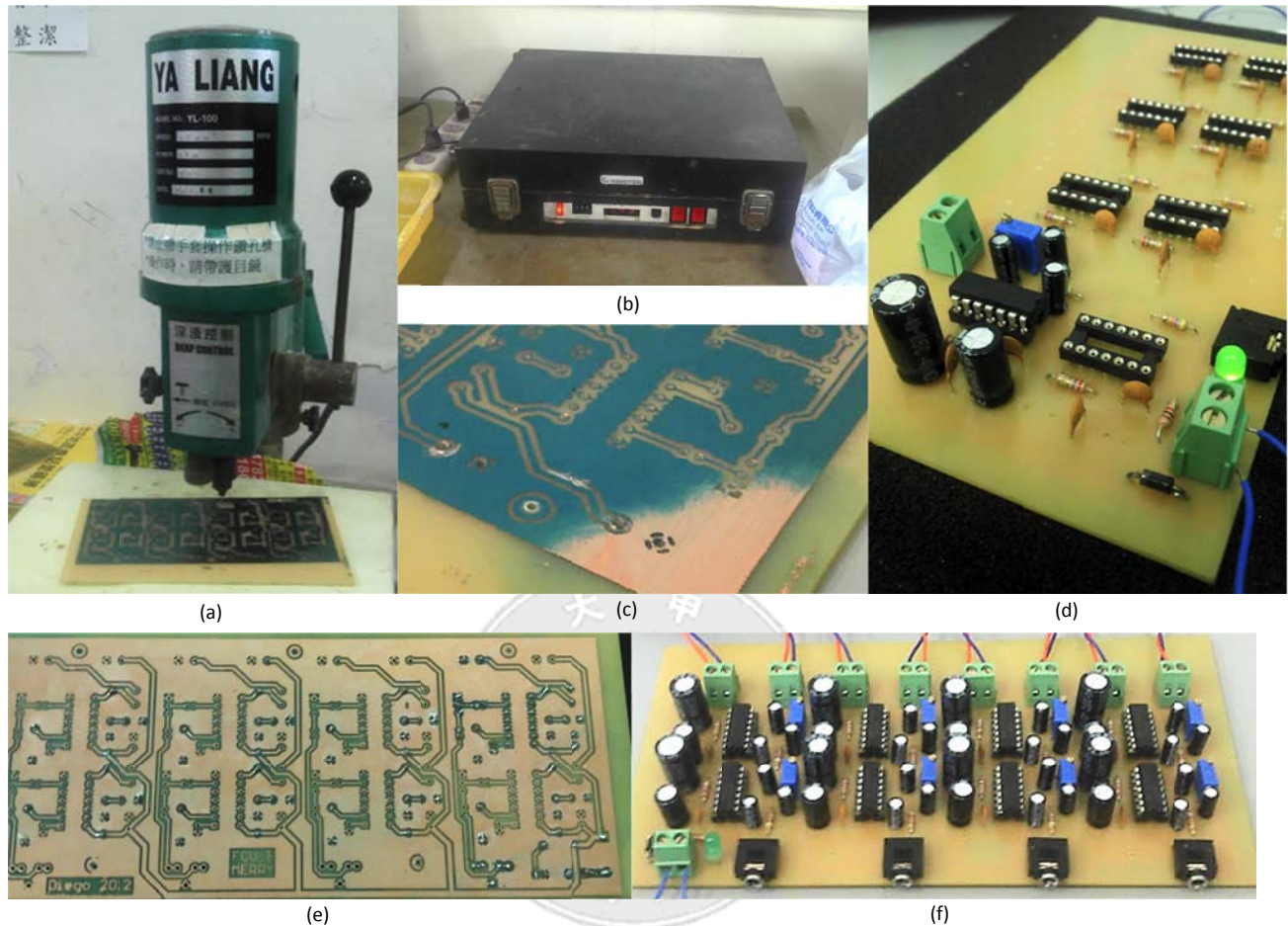
Figure 5.7 Images of the PCB construction: (a) Drilling (b) Ultra-violet enclosure (c) Placing the components (d) Cleaning photo-resist material (e) PCB without components (f) PCB with all the components
