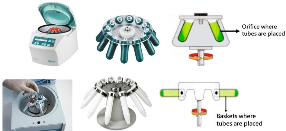
**Figure 2.** Upper row: fixed-angle centrifuge, components and tubes position during spinning. Bottom row: swinging head centrifuge, components and tubes position during spinning.
