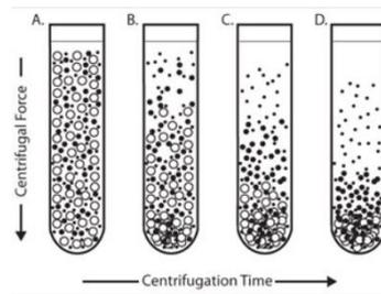
**Figure 3.** Differential centrifugation (Mark Frei, BioFiles).
