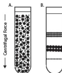
**Figure 7.** Isopycnic centrifugation (Biofiles online. Sigma.com/biofiles)
