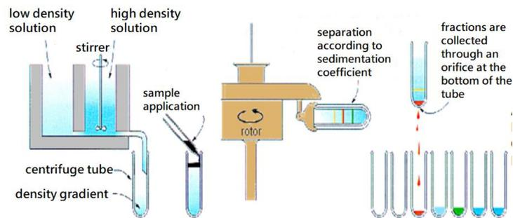
**Figure 6.** Stages of rate-zonal centrifugation. (A) Creation of a density gradient with an automatic device (B) Placing the sample on the gradient at the top of the tube (C) placing the tubes in the swinging-bucket rotor and centrifugation (D) collecting the pellets separated in bands (Source: Técnicas de laboratorio en bioquímica. Centrifugación. <http://biomodel.uah.es/>).
