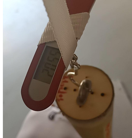
(b) Test Set up Up just before breaking under \approx 20 kg
