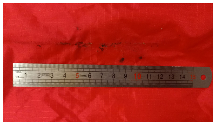
Figure 4.8: Aspera's Parachute Damage by Improper Blanket Shielding from Black Powder Charge
