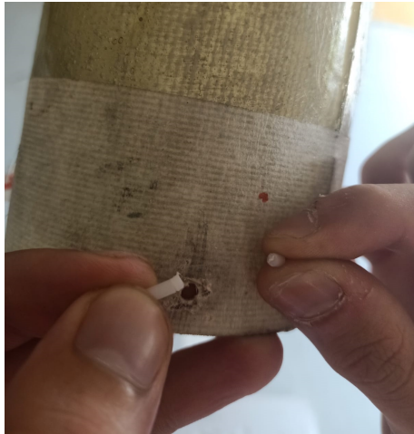
(a) Close up of Fuselage hole and broken pin
