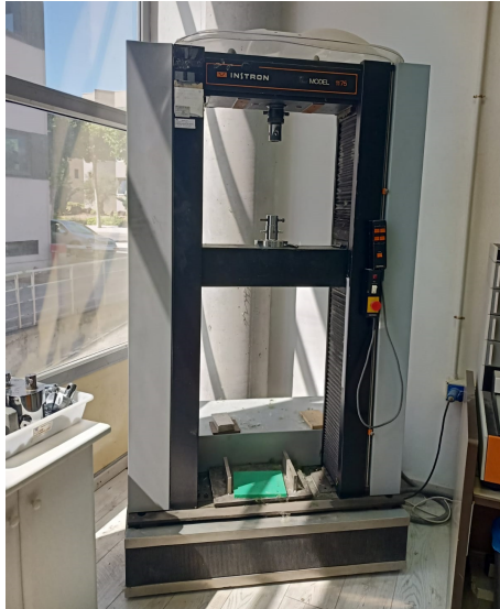
(a) Parafly's Instron ® machine used to test the breaking strength of the Kevlar slings.
