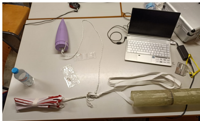
Figure 4.6: Aspera Drop Test Set Up
