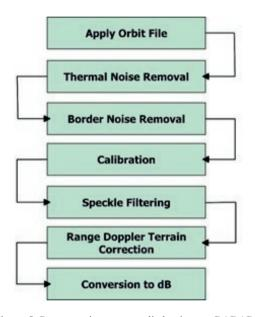
Figure 8. Preprocessing steps applied to images RADAR.
