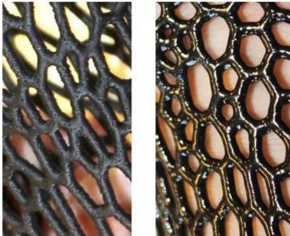
Figure 9.9. Orthosis surface before (left) and after (right) acetone post-treatment.
