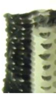
Figure 10.12. Example of an irregular profile of the deposited strands, reducing the ability to determine dimensional tolerance.
