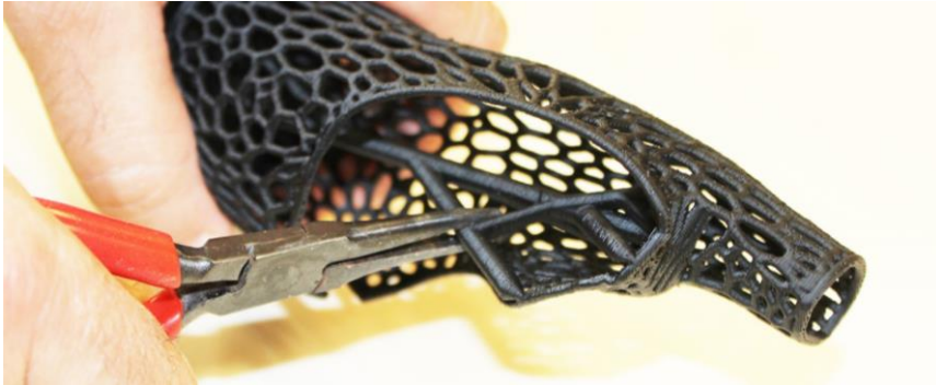
Figure 9.6. Manual removal of supports process.
