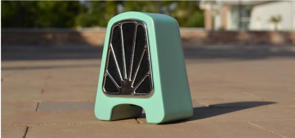
Figure 7.27. Prototype with a metallised component using vacuum PVD. Note that the deposition lines are still visible due to not enough surface preparation. Academic project from the Workshop on Prototypes and Models subject. ETSID UPV.
