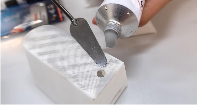
Figure 7.32. Application of nitrocellulose putty to fill gaps in a FFF component. Workshop on Prototypes and Models subject. ETSID UPV.
