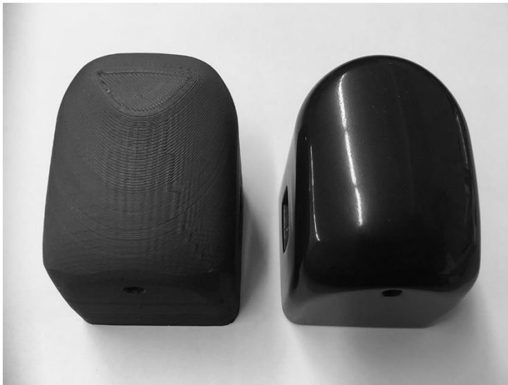
Figure 7.25. Effect of tumbling smoothing (left) and polishing (right) media in a FFF component (Schneider, 2019)
