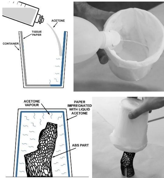
Figure 9.7. Illustration and images of the two steps of the acetone treatment.
