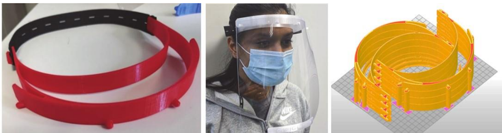
Figure 10.7. Face shield design (left), in use (centre), the stacked version for production (right).
