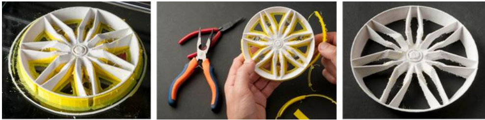
Figure 7.4. Process of manual support removal.
