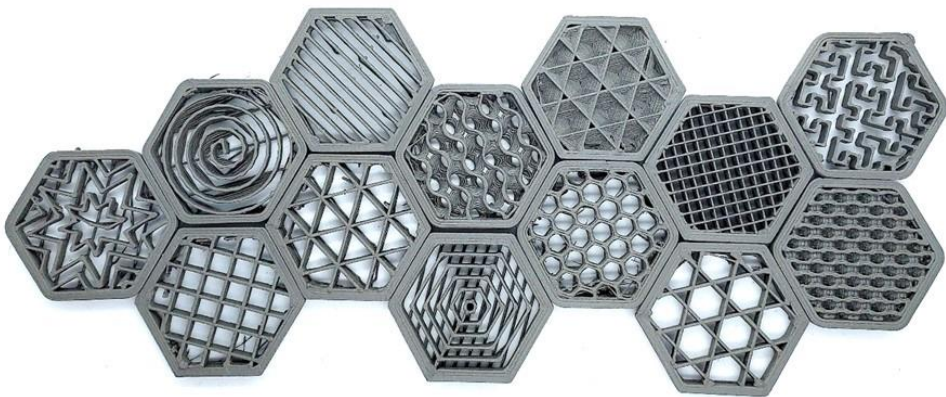
Figure 10.14. Examples of various patterns that could be used to reduce the density of FFF components.
