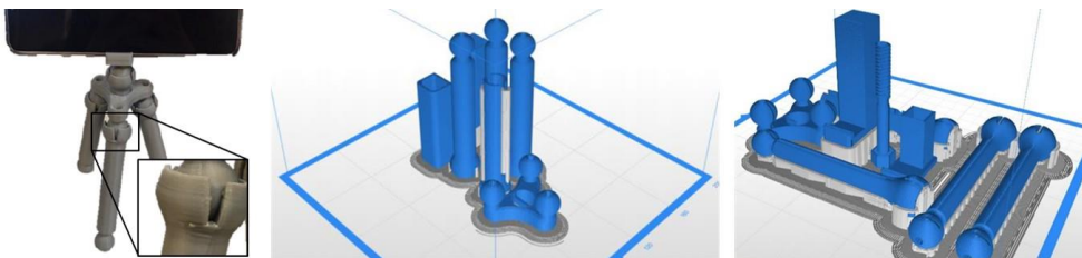
Figure 11.6. Design iterations enabled by prototyping. Problem detected (left) and orientation of the parts in the print platform (centre) and reoriented in the second iteration (right).
