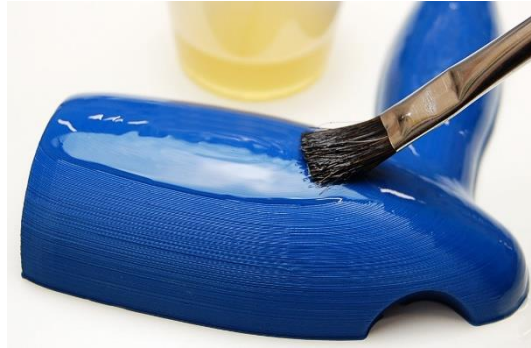
Figure 7.30. Brush application of epoxy resin to seal and smoothen the surface (BJB Enterprises, n.d.).
