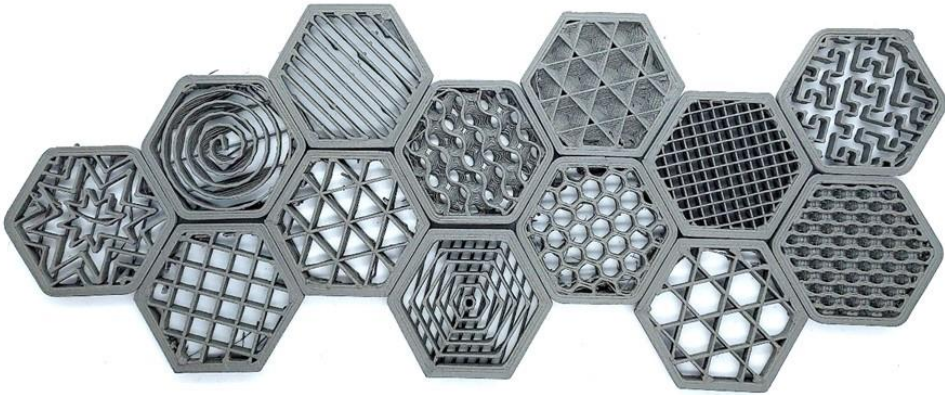
Figure 6.15. Examples of various patterns that could be used to reduce the density of FFF components.
