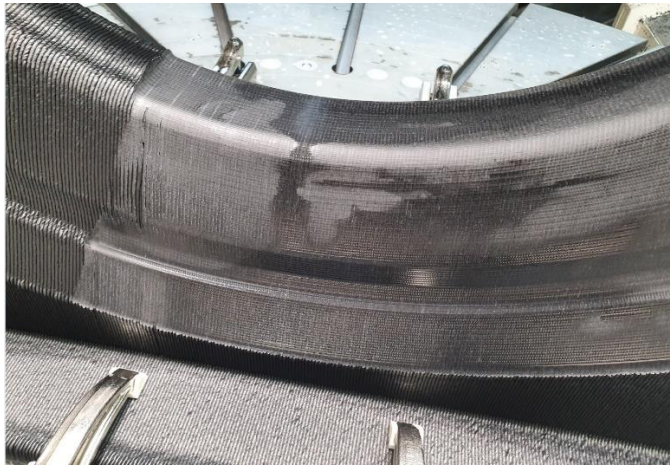
Figure 7.24. Composite mould tool being machined, produced by large-format additive material extrusion. Courtesy of The Manufacturing Technology Centre (UK).
