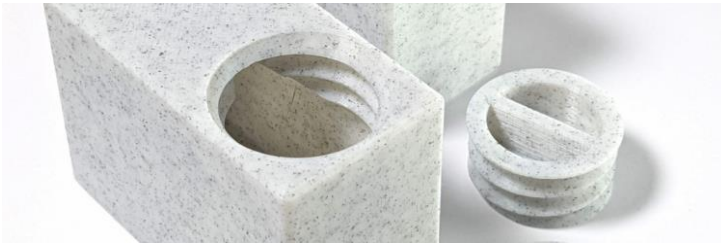
Figure 10.31. Example of FFF printed threads. Note the large size of the thread. Source: (Clockspring3D, 2020b)
