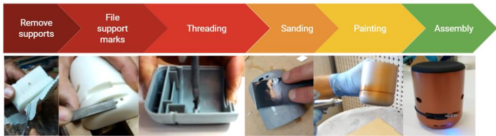
Figure 7.1. Post-processing steps of a functional FFF component.
