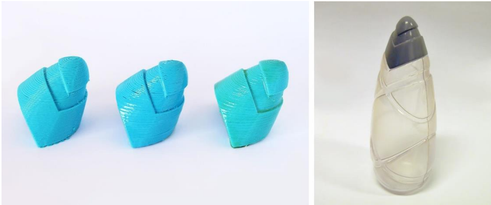
Figure 8.3. From left to right: Original 3D printed part, acetone treated, XTC-3D treated and final appearance model with traditional post-processing techniques.
