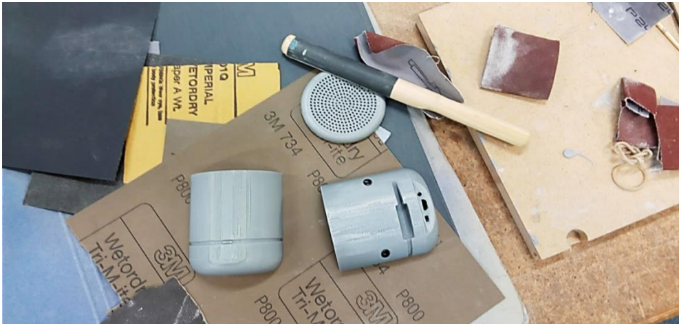
Figure 7.15. Sanding tools, including a sanding paper attached to a customised curved wooden baking tool for sanding curved areas.
