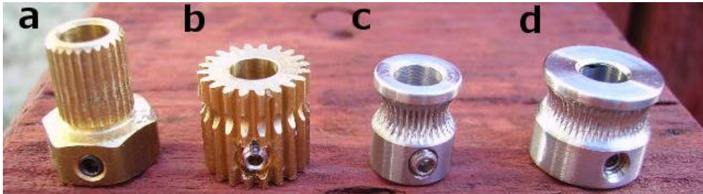
Figure 3.2. 3D Printer Extruder Filament Drive Gears: a) Plain Insert; b) Raptor Filament Drive Gear; c) MK8 Drive Gear; d) MK7 Drive Gear. Source: Airtripper.com
