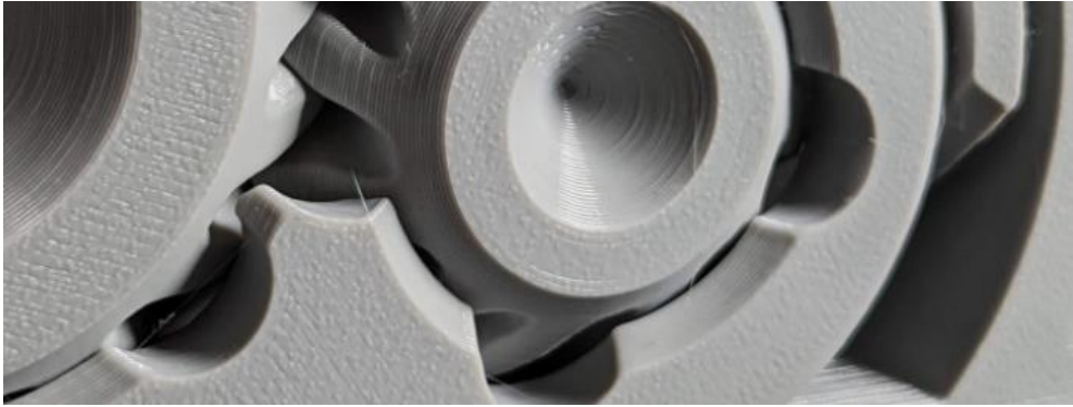
Figure 10.28. Top view of an example of clearance between moving components in a self-assembled mechanism. Source: (Clockspring3D, 2020a)
