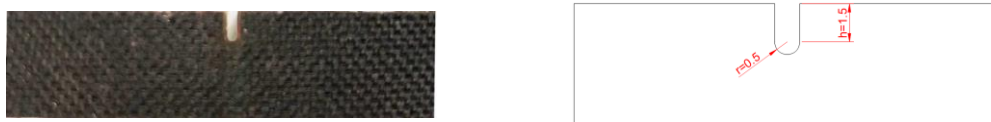
Figure III.2.5.1. Detail of U type notched samples for Charpy test to evaluate the impact strength of hybrid composite laminates with different basalt/flax plies with a partially bio-based epoxy resin.
