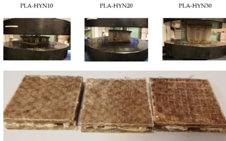
Figure III.1.3.5. Pictures of the flatwise compression test of composite sandwiches with PLA honeycomb cores with different thicknesses: The left column shows the initial elastic stage; the right column shows the image after the failure.
