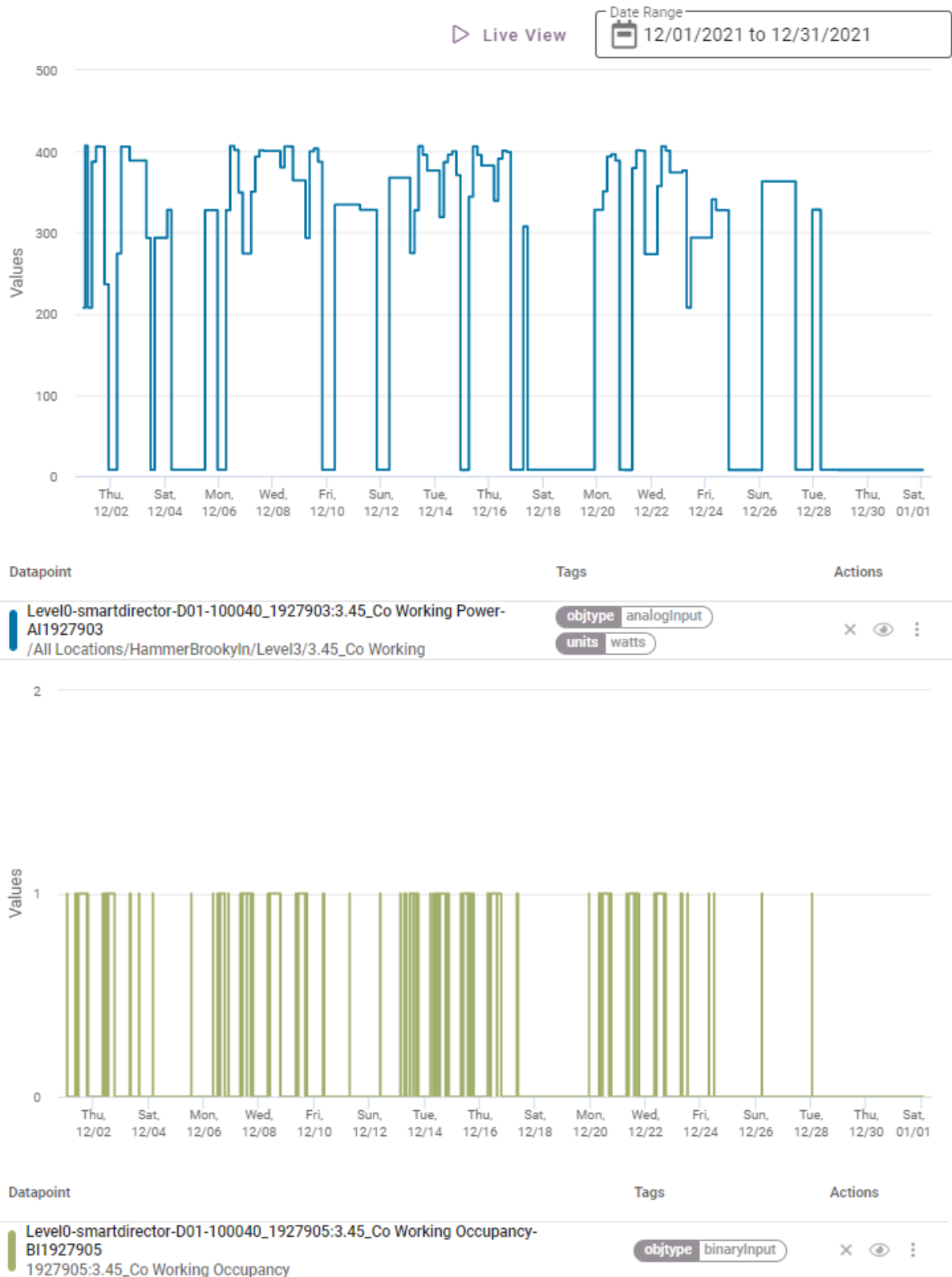
Figure A-8: Comparison of the 3.45 power state (blue) and the occupancy (green) graphically represented in the server for December 2021
