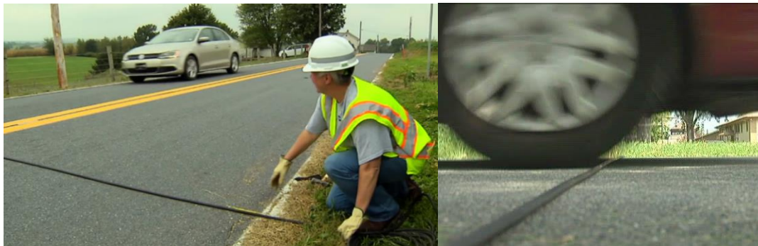
Figure 18- Image of pneumatic tube sensor working
