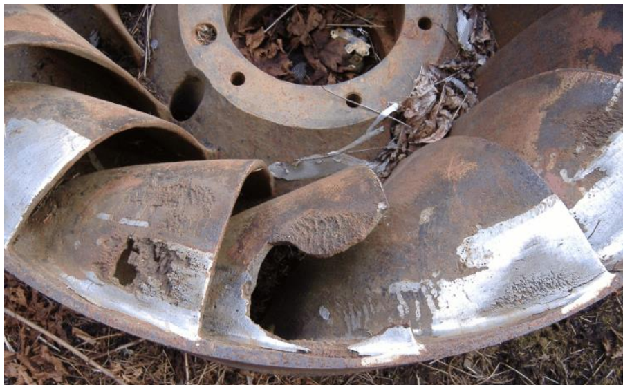
FIGURE 1.2: CAVITATION DAMAGE TO A FRANCIS TURBINE [6]
