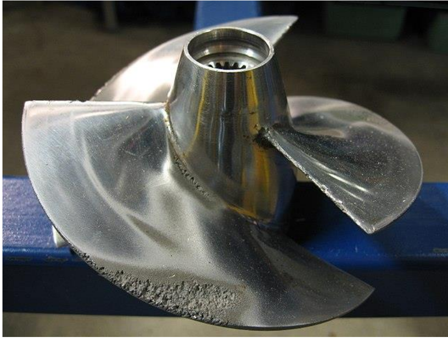
FIGURE 1.3: CAVITATION DAMAGE OF A PROPELLER [6]
