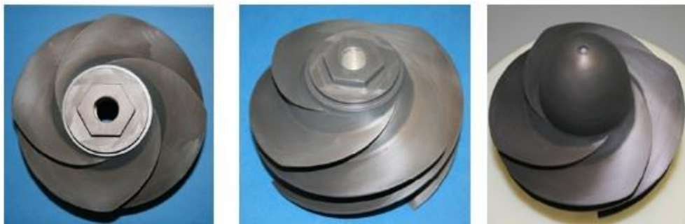
FIGURE 2.30: FRONT VIEW (LEFT), SIDE VIEW (MIDDLE) AND INDUCER WITH THE NOSE (RIGHT) OF DAPAMITO 4 [1]
