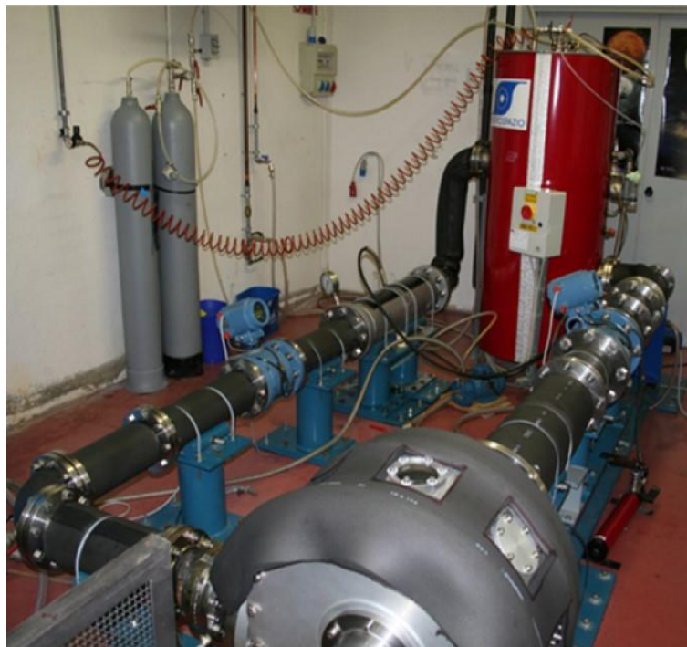
FIGURE 2.1: TYPICAL CAVITATING PUMP TEST FACILITY [1]
