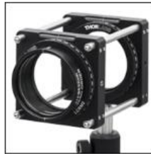
Click to Enlarge One Ø2" polarizer linearly polarizes incoming light before a Ø2" Polymer Zero-Order Wave Plate converts it to an elliptical polarization state. Each optic is mounted in an LCRM2 cage rotation mount.
