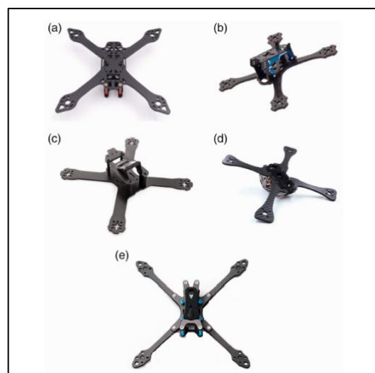
Figura 4. Symmetrical airframe models (a) HS200. (b) HS210–220. (c) HS200–210. (d) HS240. (e) HS220–230. Fuente: Castiblanco, Garcia-Nieto, Simarro, & Salcedo (2021)
