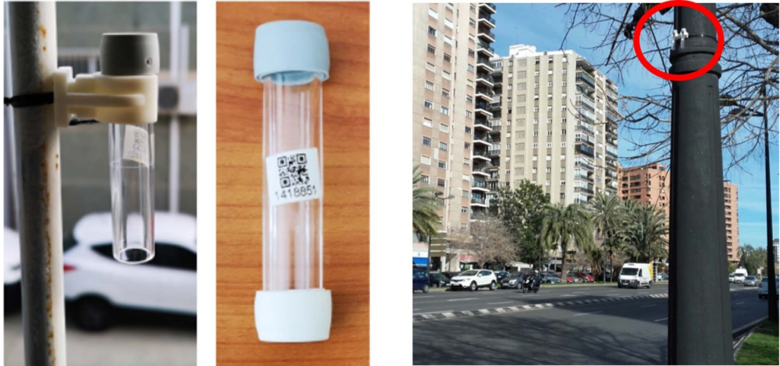
Figure 3. Left: Palmes tube to passive measurement of \text{NO}_2 ; right: north entrance and exit of the city. Photographs by José Manuel Felisi Herrero. Reproduced with permission.
