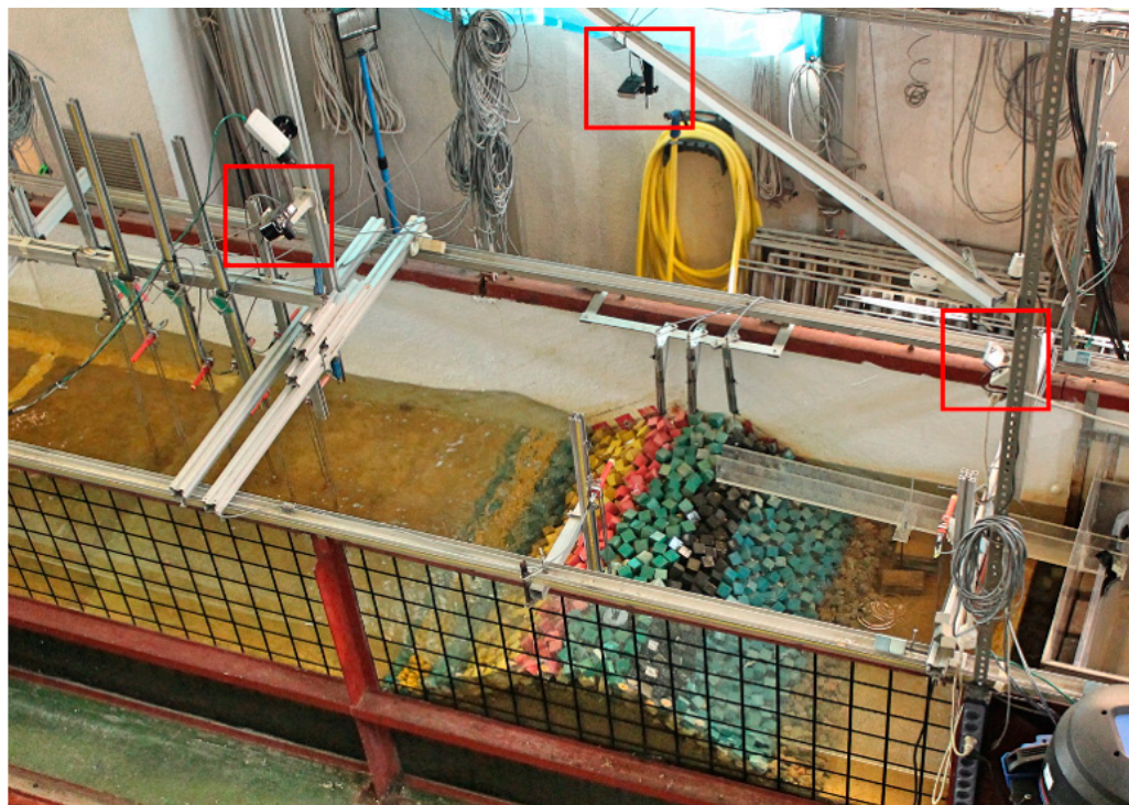
Figure 3. Location of the cameras and experimental set up for cube-armed model.
